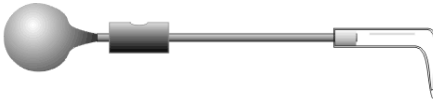
pic. 31 – a tool for applying glue
